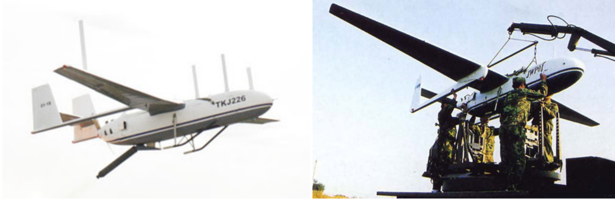
(Left: Side View of the Silver Eagle derivative of the ASN-209 with the telltale additional antenna. 53 Source: Chinese Military Review. 54 Right: Under View of ASN-209. Source: Asian Defence News. 55 )
